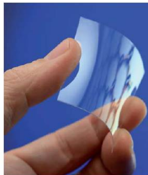
■ Figure 1.25 An experimental 'flexible' computer screen made from a sheet of graphene
