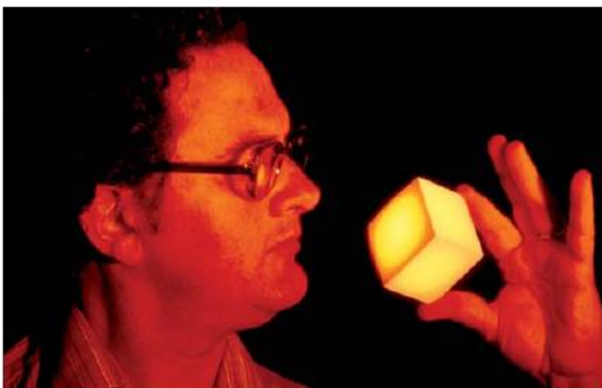
■ Figure 6.16 Metals are very good conductors of heat; other substances (such as the ceramic tiles used to protect spacecraft on re-entry) are not
