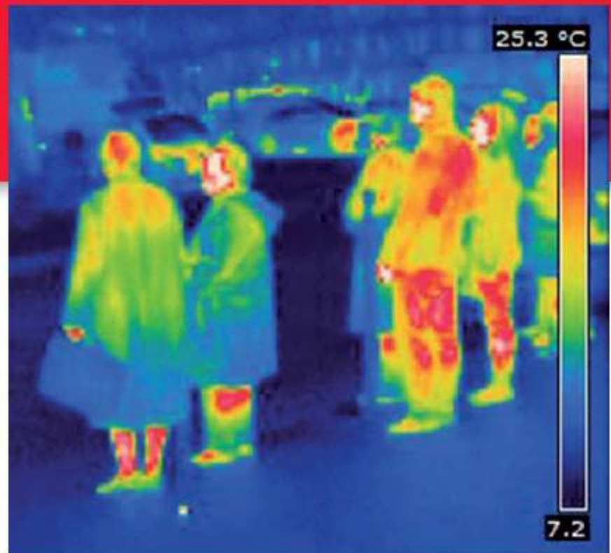
■ Figure 7.14 Infra-red topographic photograph of a human body. The colours are added artificially to represent the different intensities of infra-red radiation being released.
