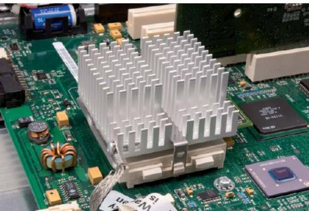
■ Figure 6.23 A heat sink is used to dissipate wasted energy as heat in a microprocessor
